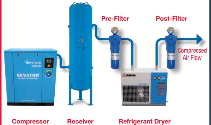
Typical Industrial Compressed Air System
