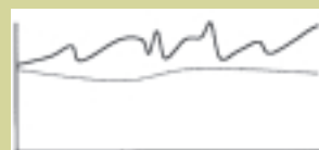
Figure 3: In situations where there is a constant load, with occasional fluctuations in demand, it may be best to use a screw compressor system for base load, with a stand-by unit to meet extra demands as they arise
